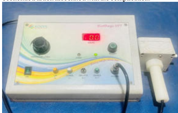
Sources: Diabetes OPD, DY Patil Hospital, Navi Mumbai Figure 1: VPT (Vibration Perception Threshold)
