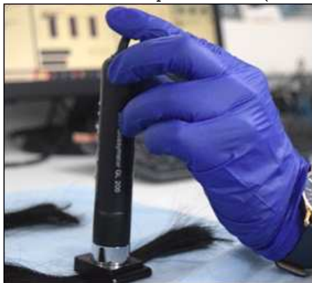
Figure 4: Hair shine assessment by Glossometer GL 200
