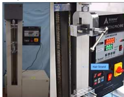
Figure 7: Tensile strength measurement using TESTRONIX
