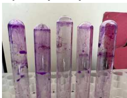
Fig.2: Biofilm adherence to glass test tube is shown by staining with 0.1% crystal violet
