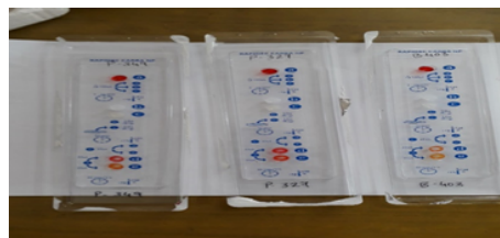
Fig.6: Rapidec Carba NP: As the colour changes from red to yellow, light orange, orange or dark orange in well e, the result is positive in right and left side but colour remains red in the middle, so it is negative
