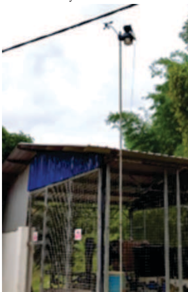
Figure 2.2: Davis Weather Station In The Durian Farm
