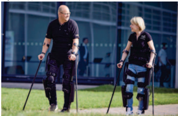
Figure 9 ReWalk rehabilitation motorized exoskeleton suit
