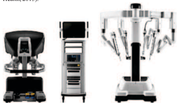
Figure 5 Left - Surgeon console Middle – Patient cart with instruments Right – The Da Vinci Surgical Robot
