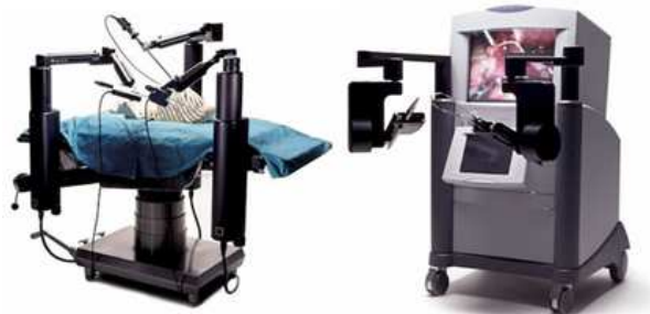
Figure 4 Left – ZEUS Robotic arms Right – ZEUS Console
