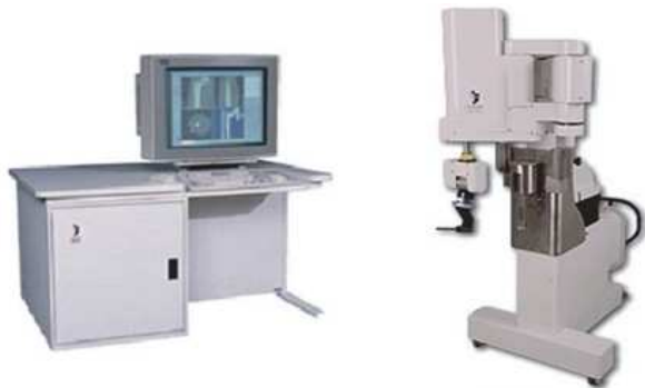
Figure 1 Left – ORTHODOC – 3D planning workstation Right – ROBODOC – Surgical assistant
