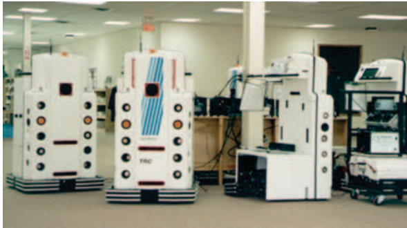
Figure 11 The HelpMate robot
