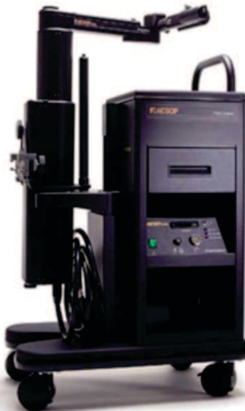
Figure 3 The AESOP Surgical Robotoperative time, neurovascular injuries, and postoperative complications (Nathan et al., 2006).
