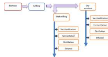
Figure2: Steps of 1G Bioethanol production from Starch containing biomasses
