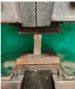
Figure no. 2: Sample mounted on the Servo hydraulic test machine
