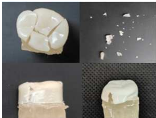
Figure no. 3: Fractured Zirconia crown, Figaro crown and Bioflx crown
