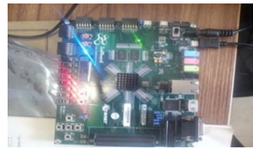
Fig 7 Hardware implementation of tpg using Gray counter Hardware : ZYNQ board, Device XC7Z020
